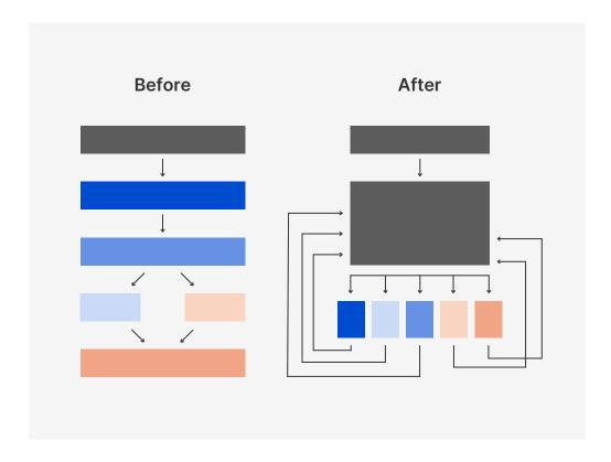
This diagram shows control flow flattening. By complicating the control flow, it makes it harder to understand where the code is going or why it takes a certain direction.
